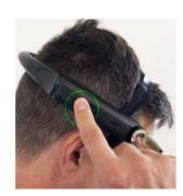
Place the display Place the display Press and hold the power close to your eyes underneath your eye in button for three seconds an upwards angle to start the device
